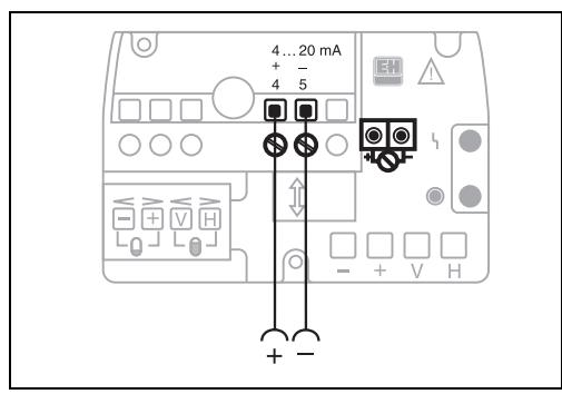
Use screened two-core instrumentation cable. For optimal protection against electromagnetic interference, the screen should be grounded in the control room or the nearest earthing point. A good connection to ground is essential to good screening.
